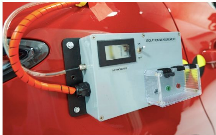
Figure 4. IIHS 305 box, showing thermocouple readout
